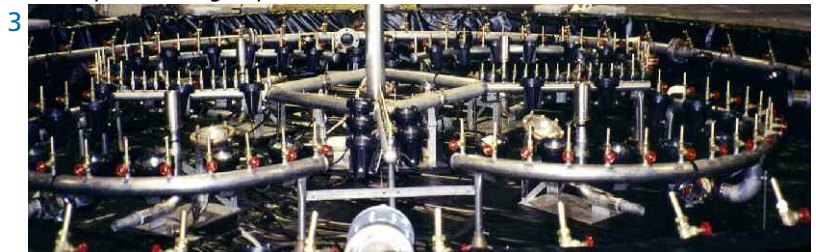
Composition des ensembles d'ajutages (FMU/FMP). Composition of groups of nozzles (UMF/PMF).
